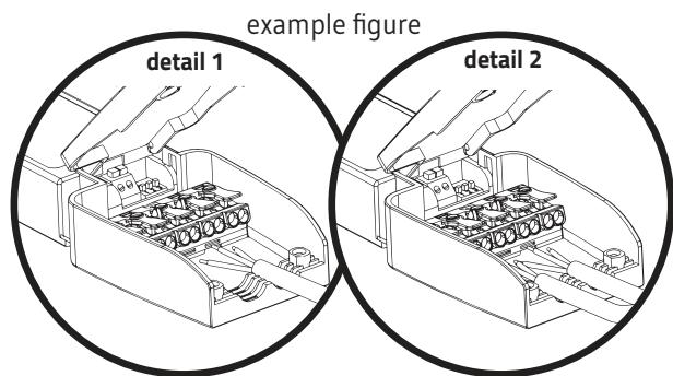
If not already present, cut out the ceiling according to the technical drawing of the corresponding GLAN model. Lay the cable according to detail 1 or 2, observing the polarity.
